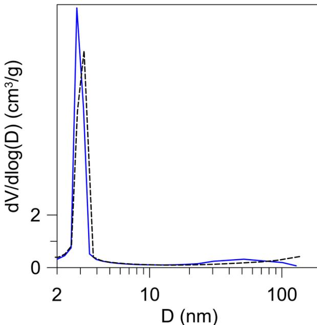
Fig. 4. The pore size distribution for MCM-41 silica calculated by BJH procedure – dash line - adsorption branch, solid line - desorption branch.
