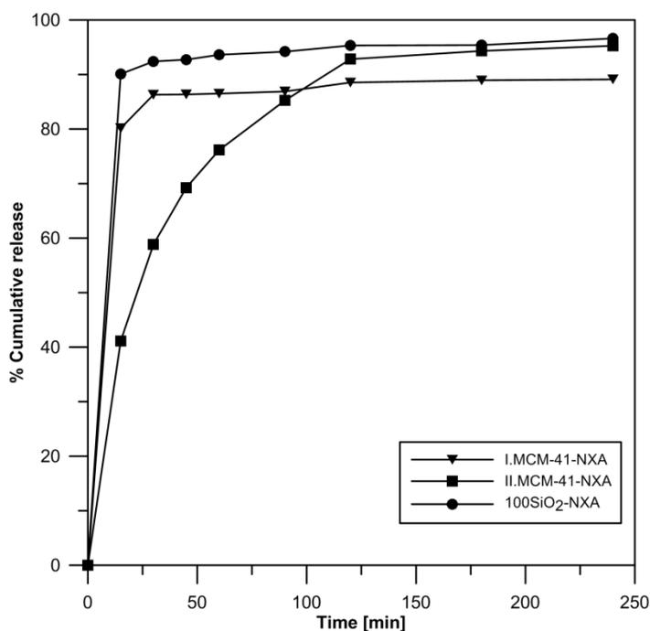
Fig. 7. Naproxen release curves from MCM-41(triangles – sample without outgassed; squares – sample with outgassed) and SiO<sub>2</sub>-100 (circles) silica material.
