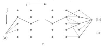
Fig. 2. The shortest path searched by dynamic programming method. The grid points represent the mesh in a 2-dimensional space  $\{x\}$  in which the functional  $S[\overline{x}]$  of Eq. (3) is defined.
