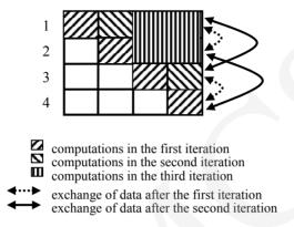
Fig. 1. Data exchange pattern for parallel Kruskal
