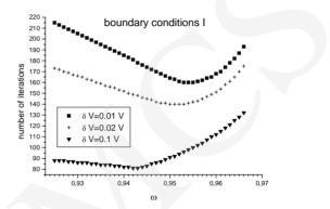
Fig. 2. Dependence of the convergence rate of the SOR method on the accuracy parameter  $\delta V$  .Results for  $V_b$ =47 V
