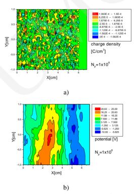
Fig. 4. Charge density and potential distribution obtained for  $10^6$  macro-particles distributed homogeneously in a rectangular box
