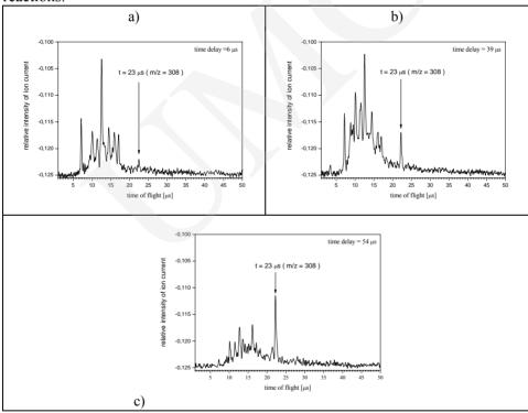
Fig. 4. Relative intensity of the ion current of 2,5-dihydroxybenzoic acid. The time delay between the laser shot and turning on the accelerating voltage: a) 6  $\mu$ s, b) 39  $\mu$ s, c) 54  $\mu$ s
