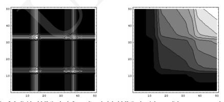
Fig. 5. Individual MI (in the left panel) and global MI (in the right panel) between two readout devices for the horizontal pattern (see. Fig 3a). 2D MI maps were generated for the first 50 ms of simulation
