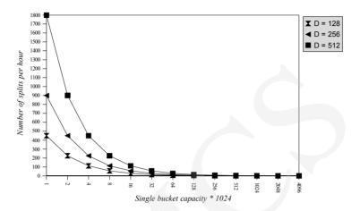
Fig. 1. The average number of bucket splits per hour considered for different bucket sizes and three data streams D
