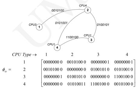
Fig.2. Example of a topology and its matrix  $\Phi = \left\| \phi_{xy} \right\|$
