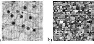
Fig. 2. Over-segmentation, (a) original image, (b) watersheds in an over-segmented image
