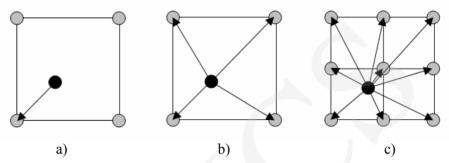
Fig. 3. The simplified schemes of charge distribution among grid points for NGP – a, CIC(2) – b and CIC(3) – c methods
