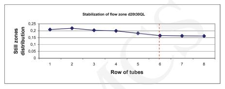
Fig. 6. Distribution of still zones area in the shell-side for square in-line arrangement  $V_L = 0.42 \text{ m/s}, V_G = 0.69 \text{ m/s}$
