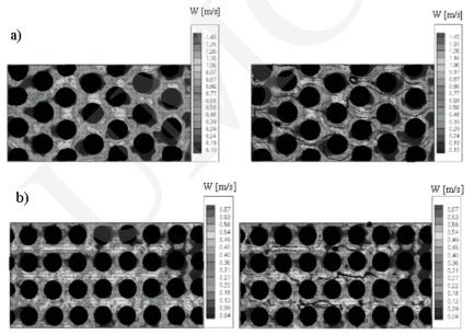
Fig. 4. Liquid velocity fields and particles motion in the shell-side (DPIV correlation algorithm), a) Triangular – staggered arrangement d20t30TS for  $V_L = 0.47$  m/s and  $V_G = 0.57$  m/s, b) Square in-line arrangement d20t30QL for  $V_L = 0.42$  m/s and  $V_G = 0.69$  m/s
