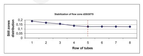
Fig. 5. Distribution of still zones area in the shell-side for traingular staggered arrangement  $V_L=0.57~\text{m/s}$  and  $V_G=0.69~\text{m/s}$
