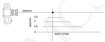
Fig. 2. Example diagram of how the f-number (aperture) affects depth-of-field
