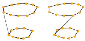
Fig 4. Contour stitching – correspondence problem. On the left side correct connection; on the right side one which could cause twisting
