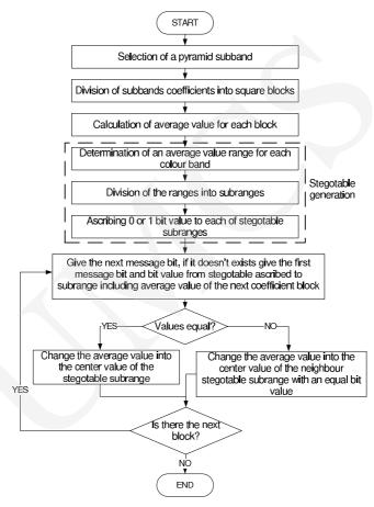
Fig. 2. Steganographic algorithm
