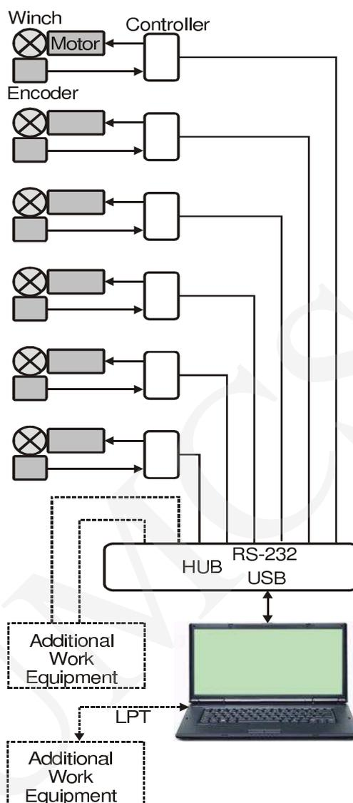
Fig. 4. Electronic system of the cable manipulator
