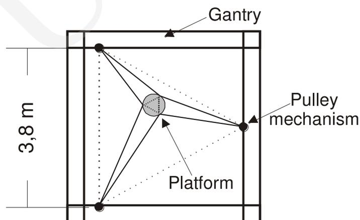
Fig. 3. Axonometric projection of the cable-driven manipulator system
