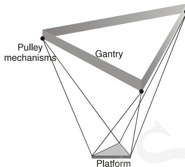
Fig. 2. Simplified scheme of the cable-driven manipulator system
