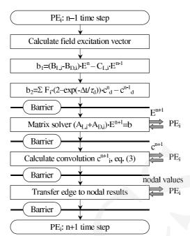
Fig. 3. Structure of tasks in the first version of the parallel algorithm
