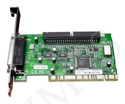
Fig. 2. Adaptec AVA 2906 controller.
