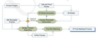
Fig. 2. Software stabilization method diagram.
