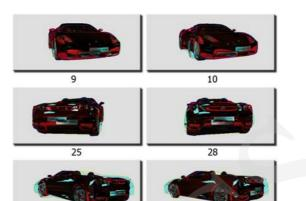
Fig. 6. Selected frames of final matching quality - difference of simulated images and aligned original photographs with the tuned parameters of position and orientation. Frames 10 and 32 are slightly mismatched.
