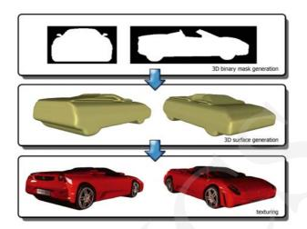
Fig. 3. Flow diagram of 3D model reconstruction algorithm.
