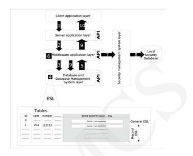
Fig. 3. The scenario of realization of the non-repudiation for user queries.
