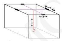
Fig. 1. The example of the conventional crane installed on the X-Y gantry.
