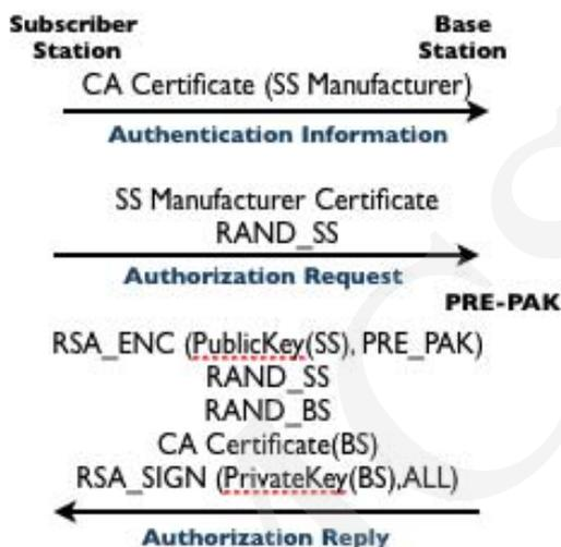
Fig. 5. Station and network authentication process in PKMv2.
