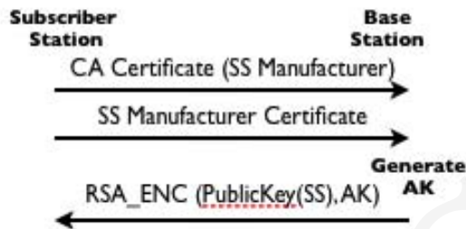
Fig. 4. Station Authentication Process.
