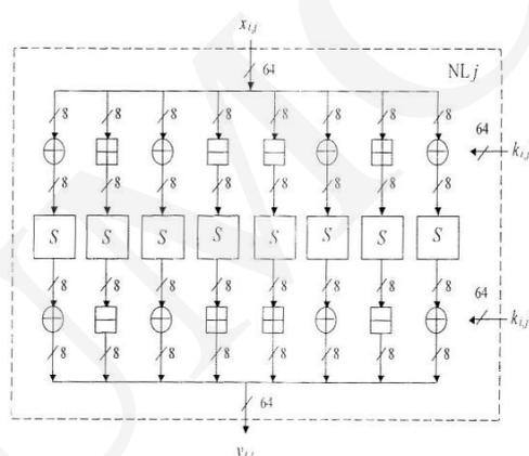
Fig. 1. Scheme of non-linear layer of PP-1 cipher.
