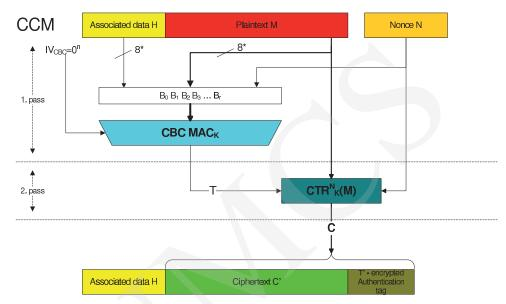
Fig. 3. CCM authenticated encryption scheme.
