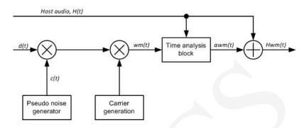
Fig. 1. Watermark embedder block diagram.
