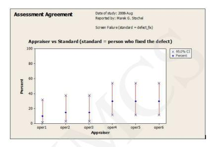
Fig. 8. Screen Failure. Assessment agreement of appraiser vs. standard (the person who fixed the defect).
