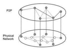
Fig. 2. Overlay network model.
