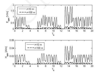
Fig. 4. Electric (top) and magnetic (bottom) fields for the 16QAM modulated signal at  $r=10\mathrm{m}$  (continuous line) and at  $r=100\mathrm{m}$  (dashed line) when  $\theta=30^{0}$ .
