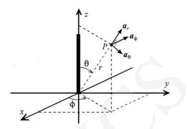
Fig. 1. A dipole of length l in the spherical coordinate. The unit vectors are  $a_r, a_\phi$  and  $a_\theta$ .
