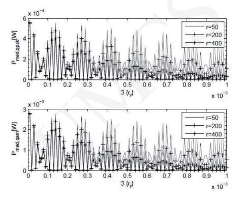
Fig. 6. Total power of the QPSK (top) and 16QAM (bottom) signals as the function of the imaginary part of the permittivity calculated at  $r=50 \mathrm{m}$  (dotted line),  $r=200 \mathrm{m}$  (line marked with '+') and at  $r=400 \mathrm{m}$  (line marked with '\*'). We considered  $\Re\{\varepsilon_r\}=6$ .
