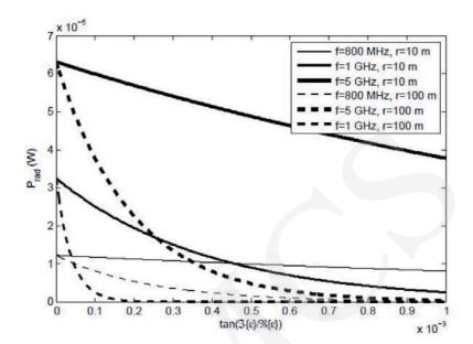
Fig. 2. The power expressed in terms of the tangent loss. We have considered the frequencies of 800 MHz (thin lines), 1 GHz (thicker lines) and 5 GHz (thicker lines) and computed the received power at r=10m (solid lines) and r=100m (dashed lines). We have considered  $\Re\{\varepsilon_r\}=6$ .
