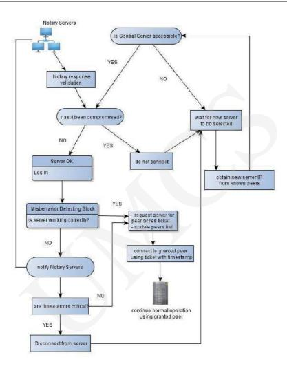
Fig. 2. Flow diagram for the user.
