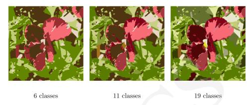
FIG. 3. Segmentations of  $flower\_3$  test image chosen based on the F and Q function values. The following parameters were used during the over-segmentation reduction – clustering method: Ward's minimum variance, watershed attributes: average and standard deviation, standard average average
