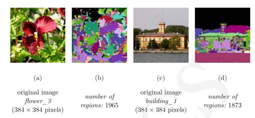
FIG. 1. The test images and their over-segmented versions. The following parameters were used for preparing the over-segmented image – flower\_3: gradient function sum-of-squares-gradient, threshold 5%, merging level 10%, building\_1: gradient function pca-gradient, threshold 0%, merging level 9%.
