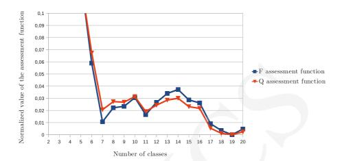
FIG. 4. Graph showing the dependence of the functions F and Q on the number of classes for the  $building\_1$  image. The function values were scaled to the interval of [0;1]. The chart shows only the [0;0,1] range in order to make local minima more visible.
