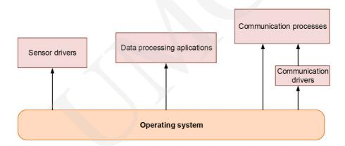
Fig. 3. Sensor software architecture model.
