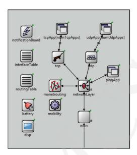
Fig. 11. Wireless sensor network node model in OMNeT++.
