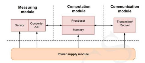
Fig. 2. Wireless sensor node architecture.
