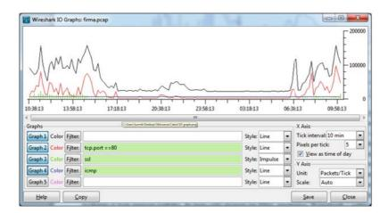
Fig. 3. 24 hours period of analyzed network traffic.
