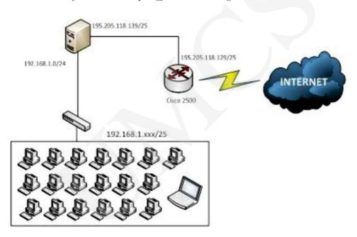
Fig. 1. Analyzed network architecture model.
