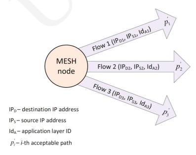
Fig. 9. Hashing Function – Load Balancing.
