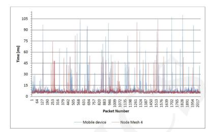
Fig. 7. Delay for packet size 1500 Bytes.
