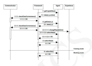
FIG. 5. Framework communication flow diagram for localization of context information gathering and processing
