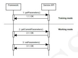
FIG. 6. Framework - Service API communication flow diagram
