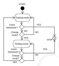
FIG. 4. Switching between Working and Training Modes
