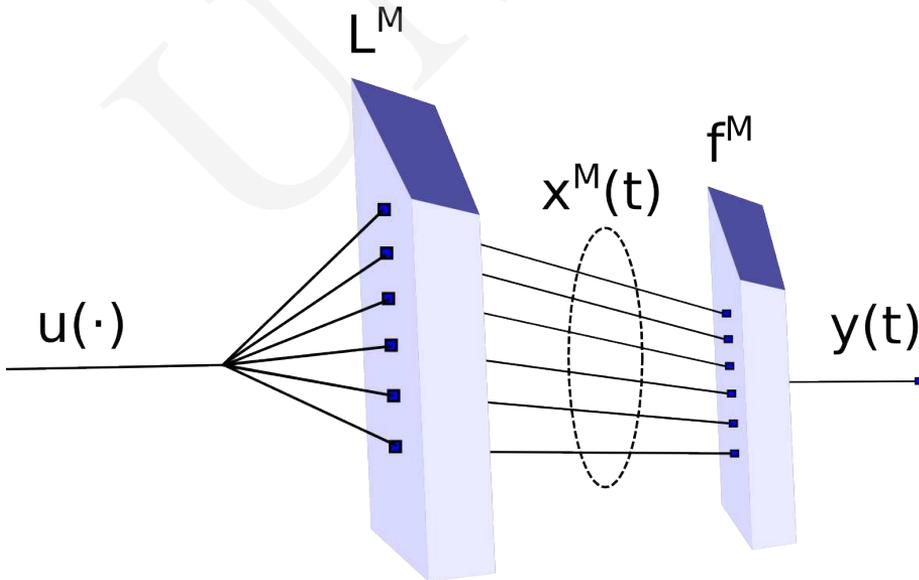
Fig. 1. The structure of the LSM
