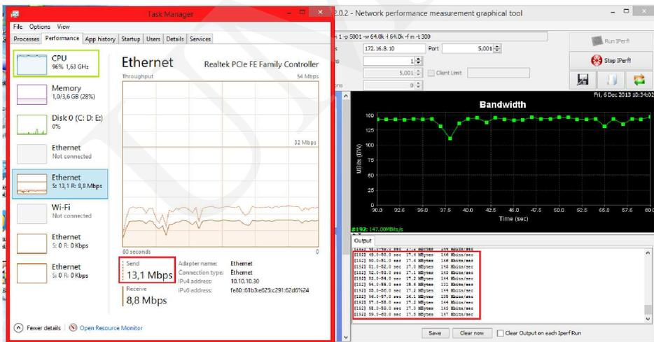
Fig. 4. 100Mbit/s link measurement with VPN tunnel.
