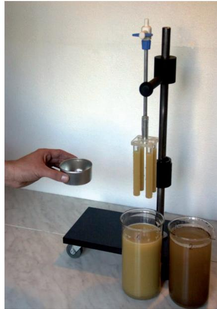
Fig. 6. A pipette with collected suspension before putting it in a weigh vessel.
