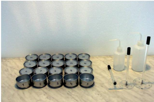
Fig. 2. Laboratory set: – weight vessels, – manual stirrers of 7 cm and 9 cm plate diameter,
