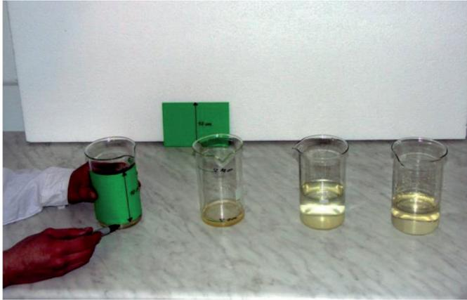
Fig. 1. Indicating “0 cm” and “10 cm” sedimentation levels on the beakers of 8 cm diameter.
