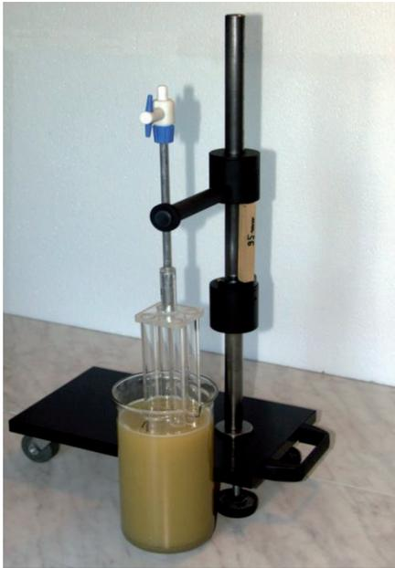
Fig. 5. A pipette lowered to the point of contact with the suspension surface; indication of pipetting depth.
